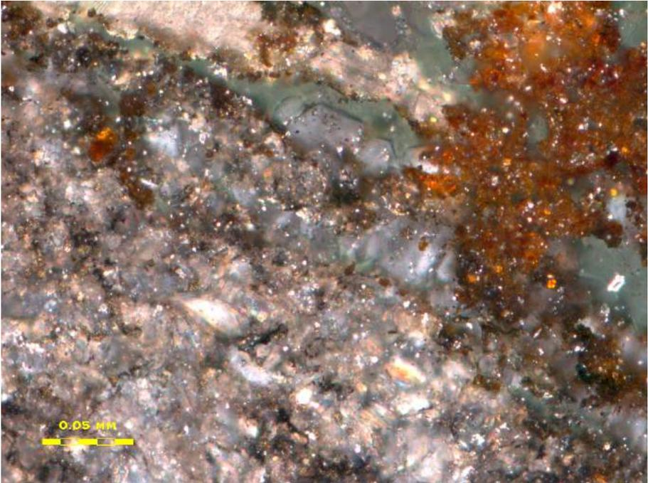
*Figure 2: Thin section, reflected light view showing muddy limestone aggregate in a concrete block exhibiting pyrite alteration and expansive gypsum formation.*
