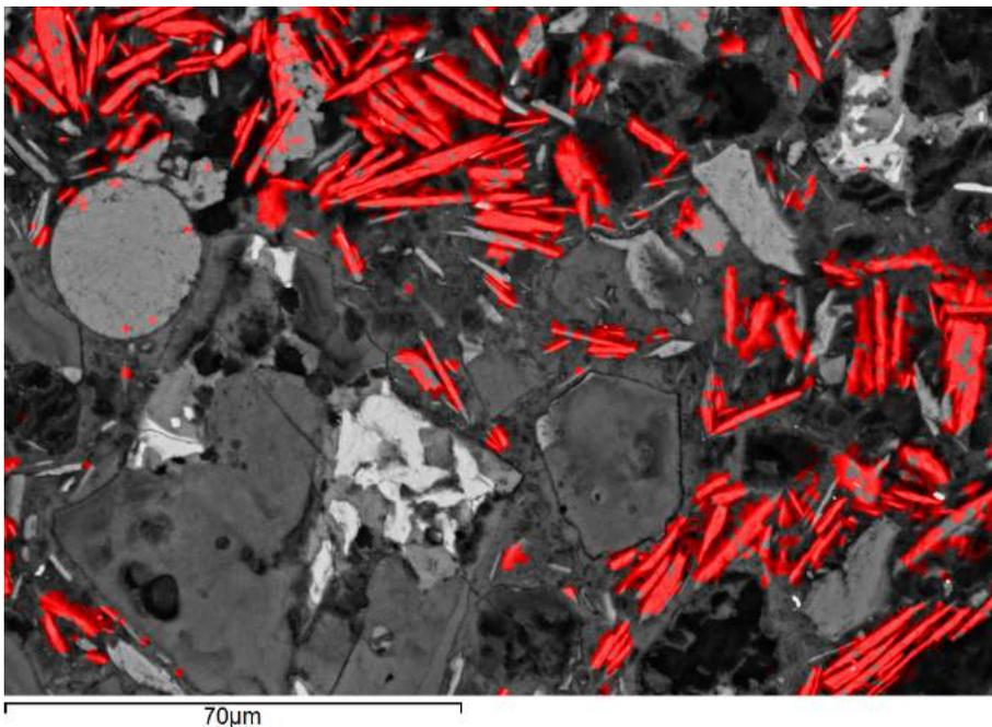
Figure 1: Phase map for muscovite superimposed on a BSE image of cement paste.
